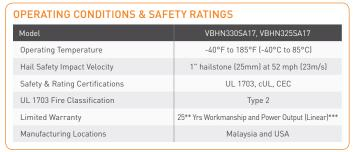
NOTE: Standard Test Conditions: Air mass 1.5; irradiance = 1000W/m²; cell temp. 25°C
