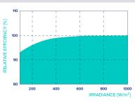
Typical module performance under low irradiance conditions in comparison to STC conditions (25 °C,  $1000 \, \text{W/m}^2$ ).
