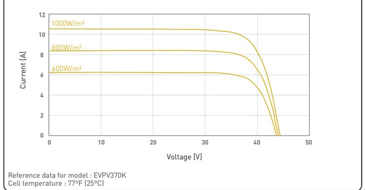
NOTE: Values at standard test conditions (STC: air mass AM1.5 irradiance 1000W/m<sup>2</sup>, temperature 25°C).
