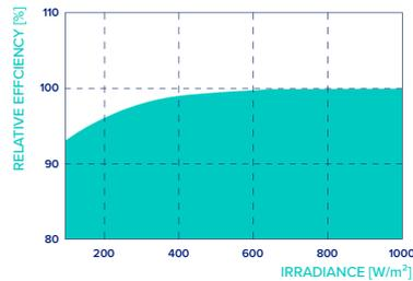
Typical module performance under low irradiance conditions in comparison to STC conditions (25°C, 1000 W/m<sup>2</sup>).
