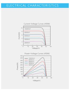
Note: the specifications are obtained under the Standard Test Conditons (STCs):  $1000 \text{ W/m}^2$  solar irradiance, 1.5 Air Mass, and cell temperature of  $25^{\circ}$ C. The NOCT is obtained under the Test Conditions:  $800 \text{ W/m}^2$ ,  $20^{\circ}$ C ambient temperature, 1m/s wind speed, AM 1.5 spectrum.
