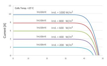
Voltage [V] Current-voltage characteristics with dependence on irradiance and module temperature
