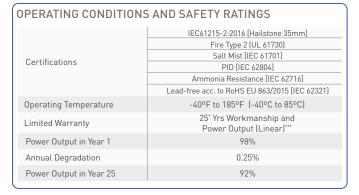
NOTE: Values at standard test conditions(STC: air mass AM1.5 irradiance 1000W/m2, temperature 25°C).
