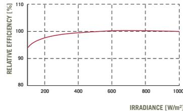
Typical module performance under low irradiance conditions in comparison to STC conditions (25 °C, 1000 W/m<sup>2</sup>).
